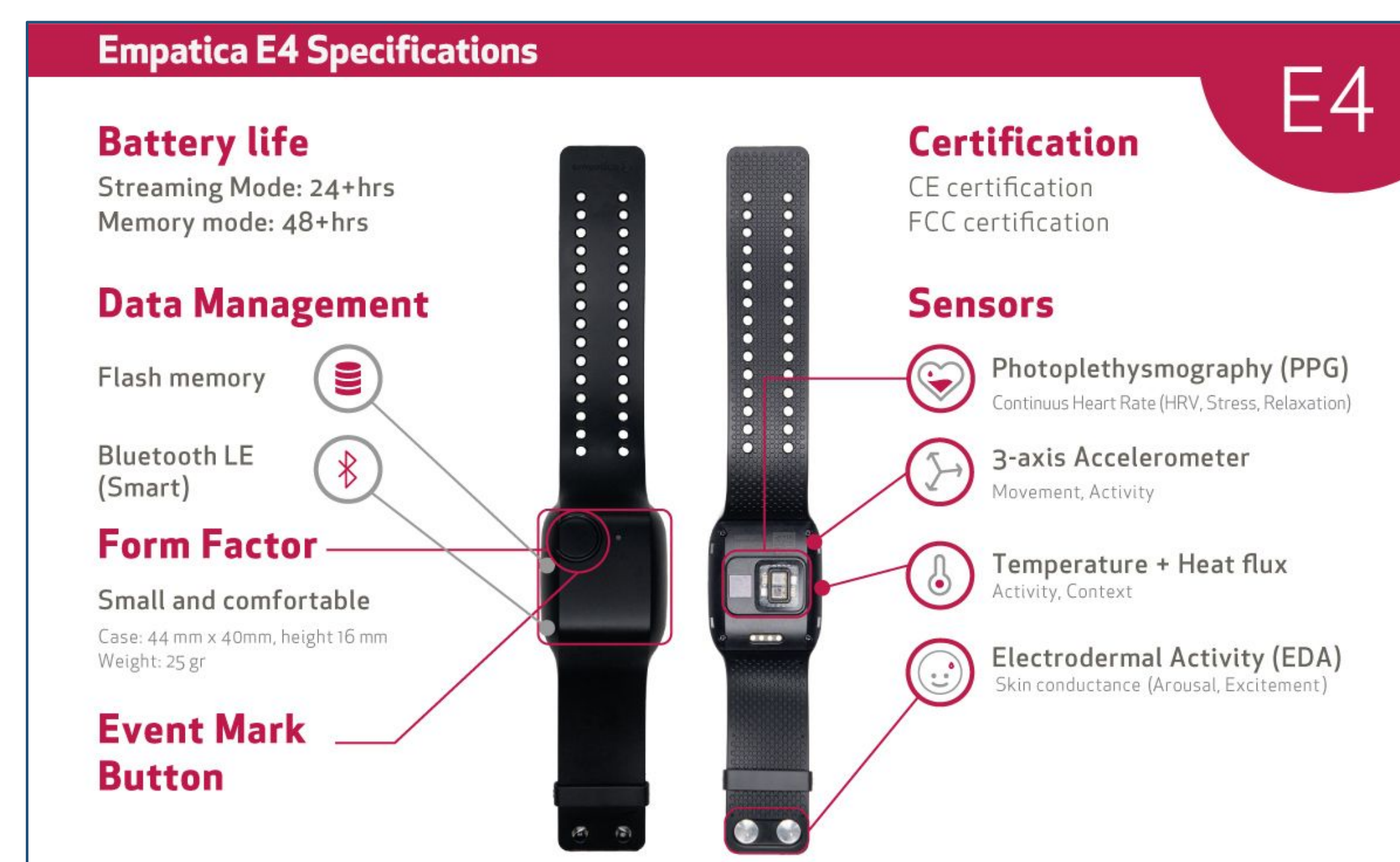
Figure 2: Empatica E4 Wristband with Core Specifications [2]
